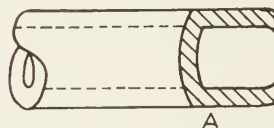
2-7. A sawing fixture used to insure square true ends when sawing tubing. (Imperial Brass Mfg. Co.)
